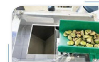
大盘负责粗给称重 Big Vibrating Hopper Is For The Main Weighing
