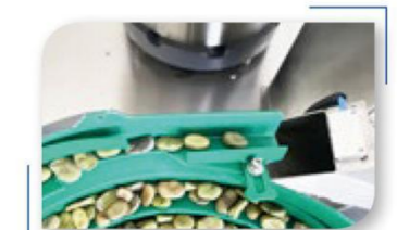
小盘负责精给计数 Small Vibrating Hopper Is For Accurate Counting
